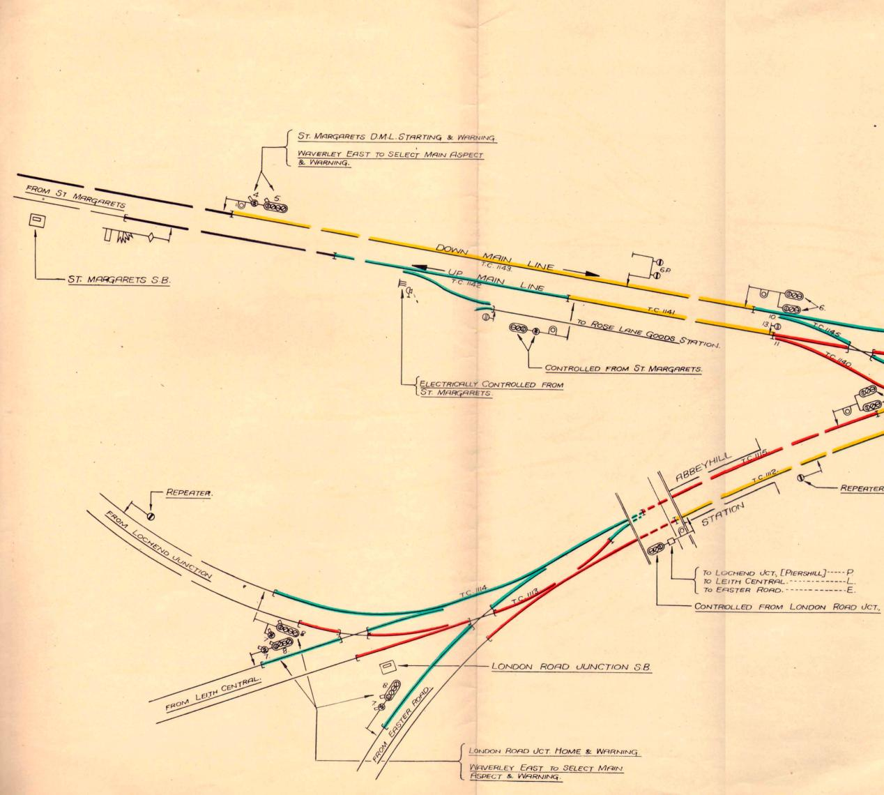
WAVERLEY EAST. DIAGRAM OF SIGNALLING ARRANGEMENTS. SPARE LEVERS \_\_\_\_\_ 1 \_\_ 2 \_\_\_ 3 \_\_\_ 19 \_\_ 22 \_\_\_ 23 \_\_\_ 27 \_\_\_ 30 \_\_\_ 43 \_\_\_ 44 \_\_\_ 82 \_\_\_ 89 \_\_\_ 97 \_\_\_ 98 \_\_\_ 138 \_\_\_ 145 \_\_\_ 168 \_\_\_ 179 . SELF ACTING CATCH POINTS. CONTRACTOR DOWN MAIN LINE SOUTH UP MAIN LINE -0 (000) CALTON NORTH DOWN MAIN LINE TO TO US TO US 1000 D LONDON ROAD JUNCTION TO SELECT MAIN ASPECT & WARNING. - SELF ACTING CATCH POINTS.
